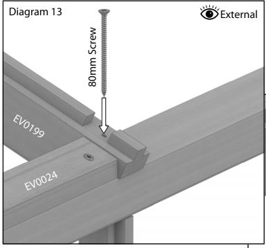
Fix the bottom of the partition roof glazing bars to the eaves bar with 80mm screws. Make sure the inside face of the glazing bar is flush with the eaves bar (shown below).
