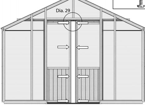
You can now install the rebate strips to the inside of your door (diagram 29). Pilot hole the strips first. It is best to do this away from the greenhouse with the 2 strips pinched together so you get the holes in the same positions. Drill 4 holes equally spaced then fix these with 40mm screws. Once the strips are in place you can fit the handles on the inside, simply line these up with the handles on the outside of the door.
