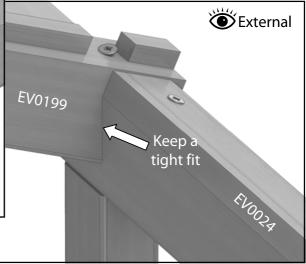
Once the bottom joint is fixed you can screw the glazing bar to the ridge (diagram 14). Do this with a 50mm screw but make sure the glazing bar is all the way into the joint. Diagram 15 shows an X-ray view of the end of the ridge. This shows the best angle for the screw. Again you want to be careful the end of the screw doesn't come through at any point.
