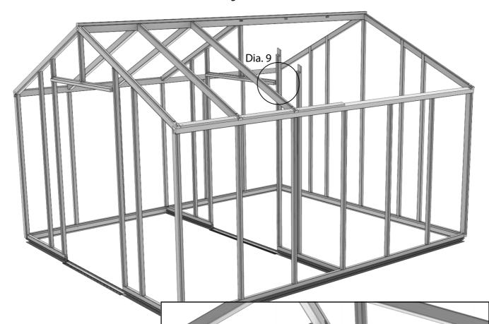
Next fit the opposite side to the aluminium base, again with two 25mm screws. With this section supported insert the door header subassembly into the mortise holes in the gable bars (diagram 9).
