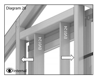
Standing on the inside of the greenhouse, with the door in the closed position you can install the door frame sides (diagram 28). Secure these with four 40mm screws per side. These should be fitted as close to the door as possible while still allowing it to pass by freely.
