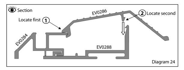
Next install the bottom door guide (EV0284) onto the door cill (EV0288) shown in diagram 24. Make sure the channels are free from grit and that this locates properly as you may find the next stage difficult if this is not the case.
