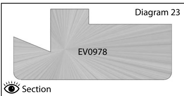
**N.B.** When you come to fixing the boarded panels either side of the door you will find there are two special capping sections (EV0978) that are slightly wider to go either side of the door.
