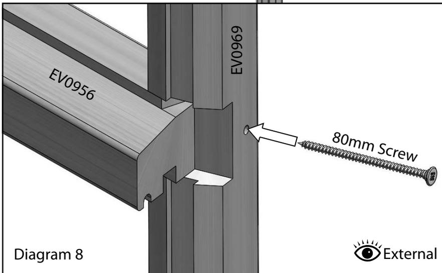
Next slot the cill into place. This is not fixed at this stage, it is secured later in the build (diagram 9). Assemble **two** identical frames like this.
